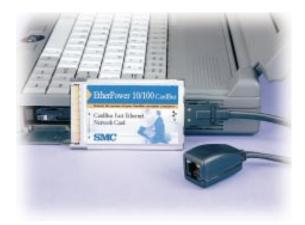
With SMC's EtherPower 10/100 CardBus PC Card, network connections have just gotten faster. This 32-bit portable PCI network card provides the quickest, easiest and most powerful way to connect to a 10 Mbps Ethernet or 100 Mbps Fast Ethernet network. And, its 100BASE-TX port supports Auto-Negotiation, so the optimum operating mode—100 or 10 Mbps and half or full duplex is selected automatically.
