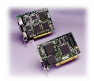
SMC's EtherPower 10/100 network cards offer the flexibility of dual-speed operation. These 32-bit PCI cards are available in two models.
