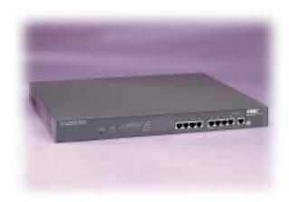
SMC's EZ Switch™ 100 is a high-performance, yet affordable, plug and play Fast Ethernet switch that is perfect for high-traffic environments. Its eight 100BASE-TX ports support Auto-Negotiation, so the optimum operating mode—100 or 10 Mbps and half or full duplex—is selected automatically for each port.
