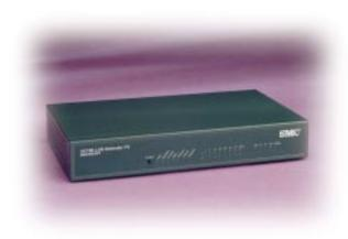
SMC's 10/100 LAN Extender FX connects an Ethernet or Fast Ethernet network to a Fast Ethernet fiber backbone. This two-port switch contains one 100BASE-TX port and one 100BASE-FX port. The 100BASE-TX port supports Auto-Negotiation, so the optimum operating mode—100 or 10 Mbps and half or full duplex—is selected automatically.
